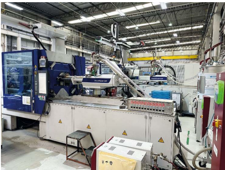
Fig. 4: Both MacroPower and SmartPower injection molding machines from WITTMANN are being used to produce headlights, rear lights, reflectors, lenses and light guides for the business segment of Automotive Lighting.
