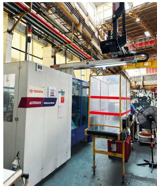
Fig. 2a+b: The glove compartments consist of two injection-molded components, a box and a lid, which are both produced on a MacroPower 650 injection molding machine with an integrated WITTMANN linear robot.
