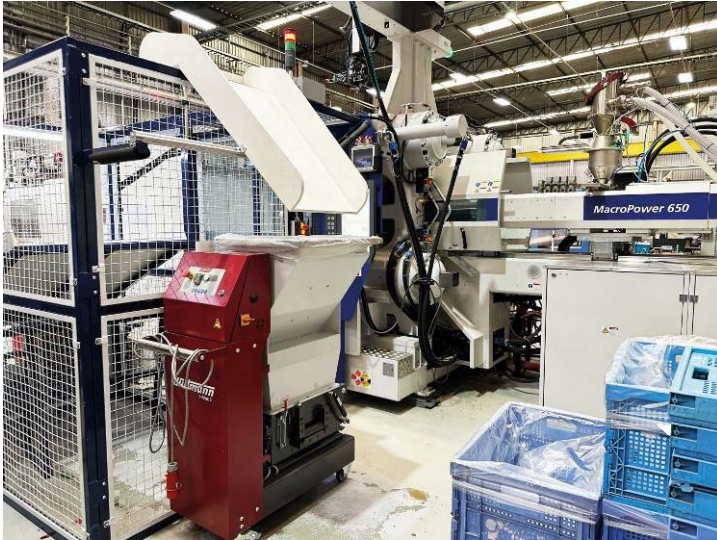
Fig. 3: Sprue is partly reground directly beside the machine and subsequently re-processed.
