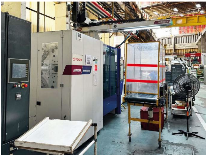
Fig. 2a+b: The glove compartments consist of two injection-molded components, a box and a lid, which are both produced on a MacroPower 650 injection molding machine with an integrated WITTMANN linear robot.
