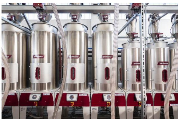
Fig. 6a+b+c: The central unit for drying and handling of the granulates supplies all of the eight injection molding machines with a wide range of materials. (Photo: ZECA)
