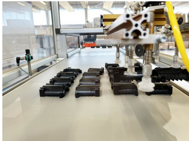
Fig. 9a+b: The handle pieces made of PC-ABS are produced in two halves inside a 2+2-cavity mold. (Photo: WITTMANN)
