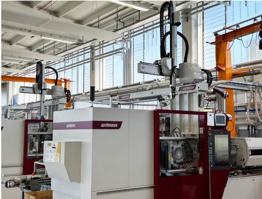
Fig. 8: All injection molding machines are equipped with linear robots from WITTMANN. (Photo: WITTMANN)
