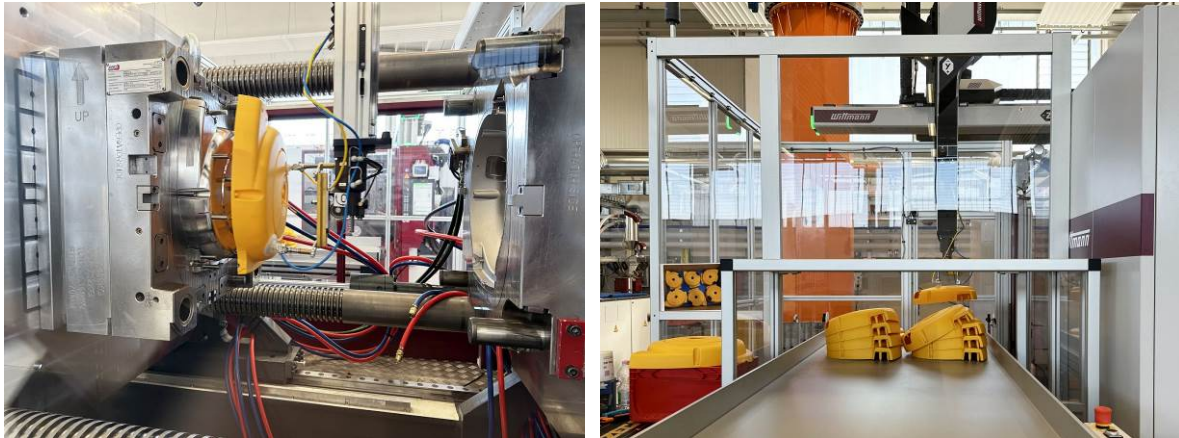
Fig. 10a+b: The housings for cable and hose reel systems made of PP are currently among the largest parts produced on MacroPower machines. (Photo: WITTMANN)
