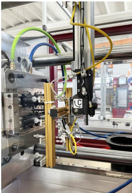
Fig. 9a+b: The handle pieces made of PC-ABS are produced in two halves inside a 2+2-cavity mold. (Photo: WITTMANN)
