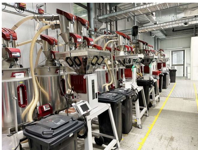
Fig. 4a+b: The granulate is fed into the materials handling system with gram-accurate precision by Gravimax gravimetric blenders from WITTMANN.
