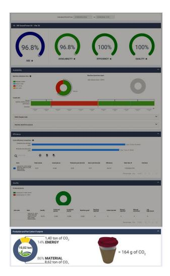
The TEMI+ dashboard shows the product carbon footprint at a glance and indicates the share of the injection molding process and the share of the material in the total emissions.
