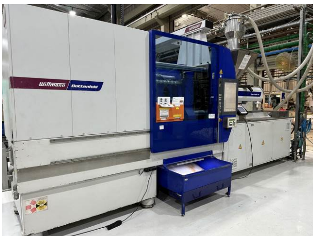
Fig. 8: For the production of fitting components with metal threading, the WITTMANN team developed a new, fully automatic production process based on a SmartPower injection molding machine.
