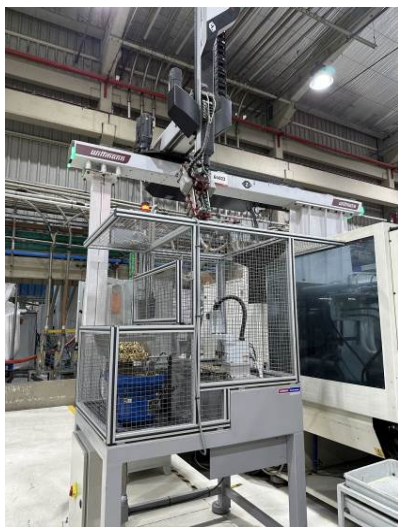
Fig. 9: The automation cell for separating and feeding the metal threads was specially designed and produced by WITTMANN BATTENFELD do Brasil as a customized solution for Krona.
