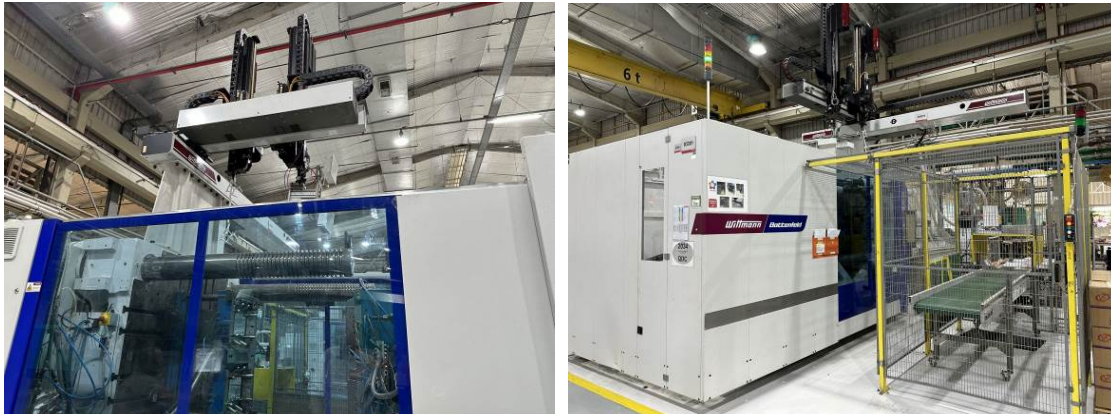
Fig. 6a+b: Customized solutions: for Krona, WITTMANN BATTENFELD do Brasil developed application-specific automation equipment, such as a two-armed linear robot.
