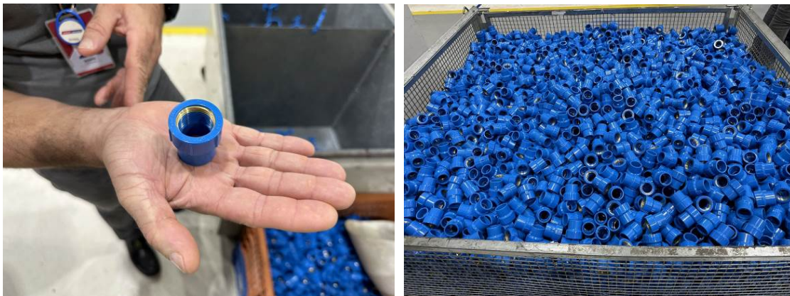
Fig. 7a+b: In the fittings sector, metal inserts are frequently over molded.
